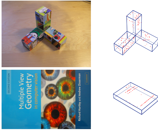
Figure 5. Real data set models. 3D models (Right) of real objects were created manually and image textures (Left) were mapped on the models. Red dots show feature points detected in the textures.
