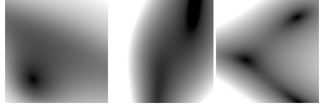
Figure 3. Qualitative distribution of homography mapping error (length of error vector) in a sample image, black means low error while white means large error. Left: The homography mapping error is low near the affine feature and increases outwards (result from extrapolation). Center: In the 2-point algorithm the error can have two local minima near the two feature positions. Right: Error for DLT on 4 point correspondences. \sigma was 0.5 pixels and principal point distortion for 2-point was 1 degree.
