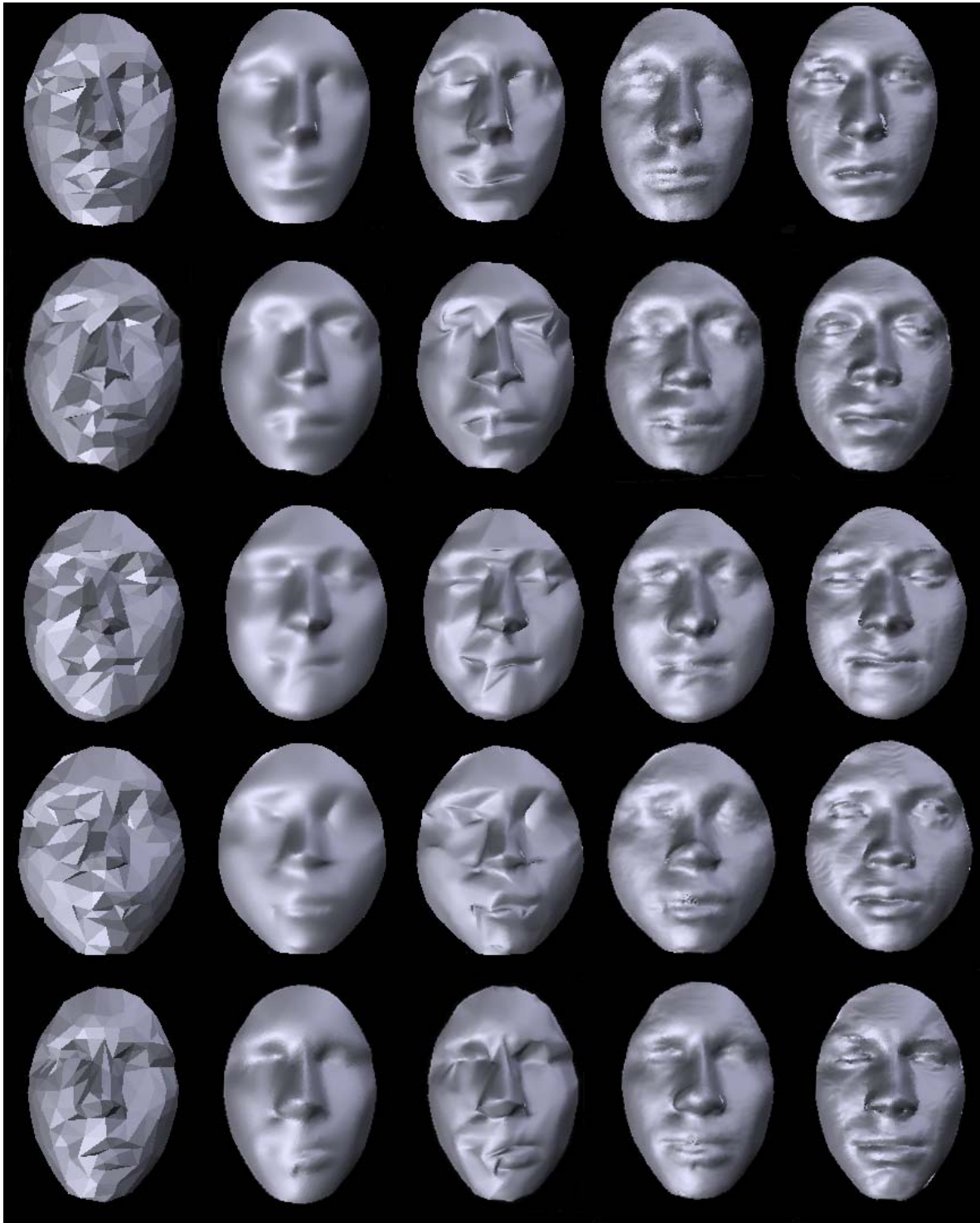
Figure 7. Hallucinating results and comparisons. (a) The input low resolution meshes, each with 150 vertices, (b) Loop's subdivision, (c) Subdivision by 3D Max , (d) Our hallucinating result, (e) The original high resolution meshes.
