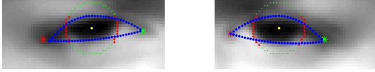
Figure 5. Eye corners are represented with an asterisk. The iris is shown as a circle, of which, the red part is the visible component. The upper and lower contours of the shape of the eye are shown in blue.
