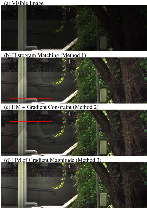
Figure 6. Comparison of Methods 1, 2, and 3. Note that the band-effects (regions in red box) due to blind histogram matching have been successfully suppressed by our guided histogram matching of gradient magnitude. The result of Method 3 achieves the least artifacts and best perceptual quality.
