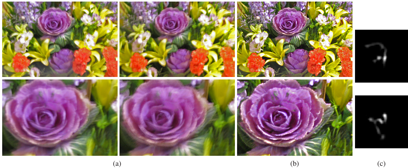
Figure 11. Deblurring FLOWER photos. (a) Two blurred inputs. (b) Deblurred result using the proposed approach. (c) Estimated kernels. Kernel size is 49 by 49.
