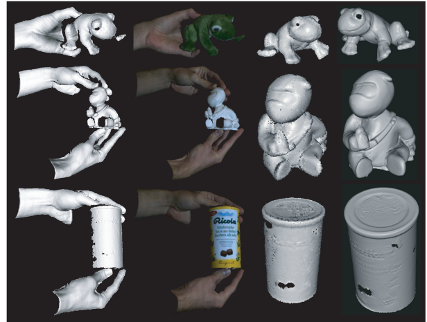
Figure 1. In-hand modeling of different objects: Typical scan, textured scan, online preview model and final post-processed model for frog , boris and ricola .
