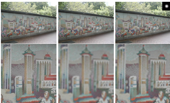
Figure 9. 4x Super-Resolution. (left) The original image and zoom-in, (middle) the original image bi-cubically downsampled and re-upsampled by 4x and zoom-in, (right) the upsampled image deconvolved using the recovered 4x super-resolved kernel (displayed in the top right of the image—the kernel has been enlarged by 10x for display) and a zoom-in on the bottom.
