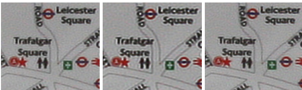
Figure 6. Kernel Size and Orientation. Image deconvolved with (left) our kernel, (middle) our kernel scaled 20% larger, and (right) our kernel rotated by 45^\circ . The middle and right images have more ringing (most apparent at the bottom of the word “Leicester”).
