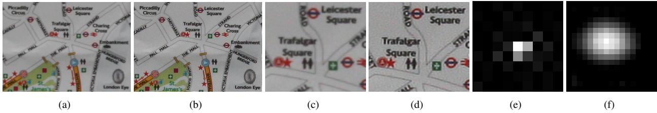
Figure 5. Defocus and Slight Motion-Blur. (a) The original blurred image and (b) the deconvolved output using our recovered PSF. (c–d) Zoomed-in versions of the original and deconvolved image respectively. (e) The kernel recovered using the method of Fergus et al. [3] and (f) our recovered kernel.
