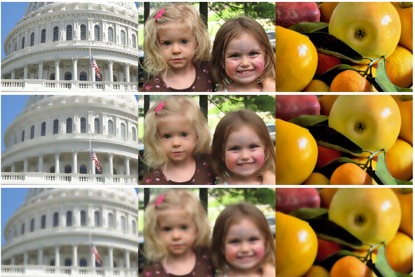
Figure 9. Top Original color images. Middle O(1) ArBs bilateral with box spatial and Gaussian range ( \sigma_r^2 = 0.05 , f : 21 \times 21 ). PSNR is 50.61dB. Bottom O(1) GrAs bilateral with Gaussian spatial ( \sigma_s^2 = 1 , f : 10 ) and Gaussian range ( \sigma_r^2 = 0.13 ). PSNR is 55.12dB. Images are 1 MB. Each channel is processed independently.
