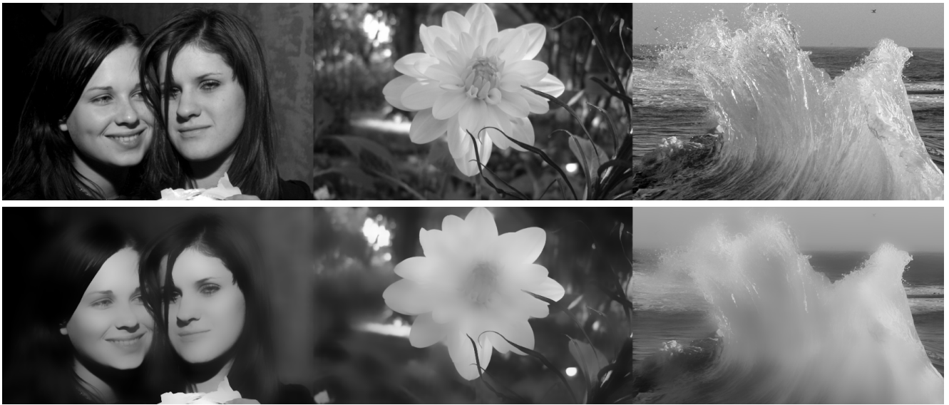
Figure 7. Top Original images. Bottom O(1) ArBs bilateral with box spatial and Gaussian range ( \sigma_r^2 = 0.15 , f : 31 \times 31 ). PSNR is 301.88dB (i.e. almost identical to the exact filter result). Images are 1 MB.
