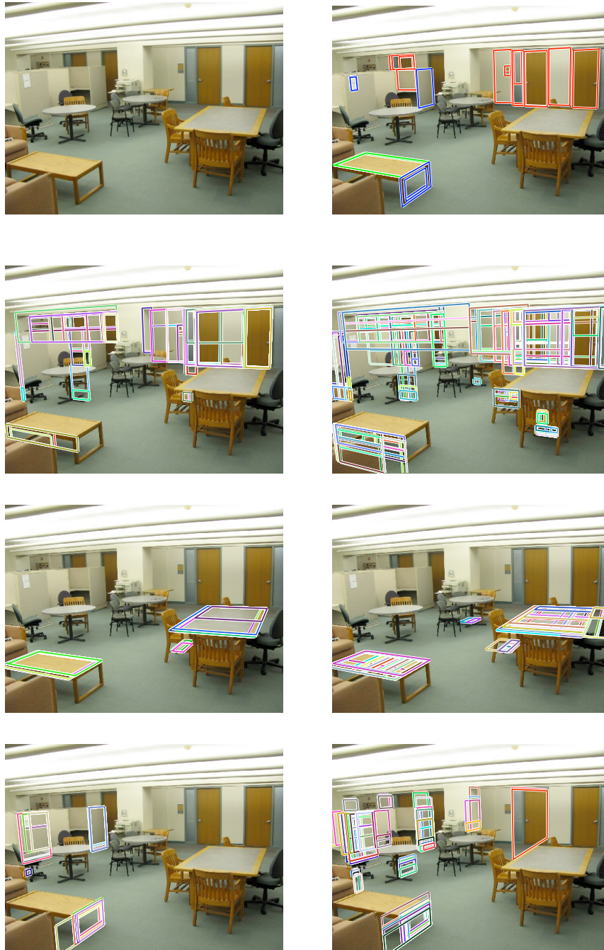
Figure 1. Rectangle detection results. The following explanation applies to all figures in this document. First row: Original image and complete rectangles detected in the dominant orthogonal planes. Second to last row: Closed incomplete rectangles (left column) and closed U-shapes (right column).
