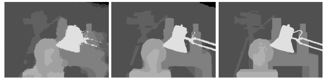
Figure 6. An application of our multi-view denoising algorithm for depth estimation. Left: the depth map estimated from the 25 noisy Ohta images. Middle: the depth map estimated from the 25 denoised images produced by our denoising algorithm. In both cases, the depth maps are estimated using graph cuts [11]. Right: the ground truth depth map. The error rate is defined as the percentage of the pixels with over one disparity difference compared to the ground truth. The benefit of using our algorithm for depth estimation is clear.
