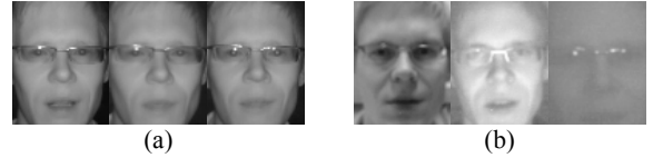
Fig. 7. Faces captured under different illuminations; (a) images under NIR condition with the three environmental illuminations: normal, weak and dark (from left to right); (b) images under three different VIS conditions: normal, weak and dark (from left to right).
