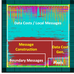
Figure 8. The floorplan of the developed VLSI circuit.
