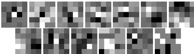
Figure 3. The thirteen 5 \times 5 FOE filters trained using our approach for the level of noise \sigma = 20 and for a three iteration ( n_{iter} = 3 ) steepest descent inference algorithm.
