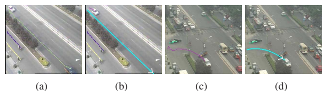
Figure 3. Examples of trajectory fitting. The white arrows are the moving directions of objects. (a) and (c): The trajectories in scene S1 and S2 respectively. (b) and (d): The results of trajectory fitting.
