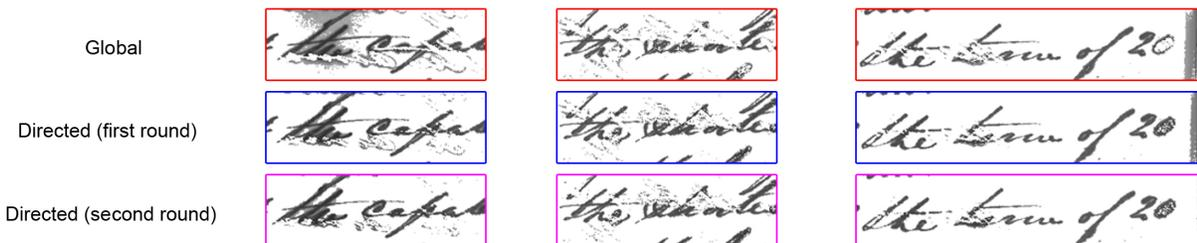
Figure 8. Three rounds of markup applied on a difficult example with strong ink-bleed. The first global markup results in a large amount of low-confidence pixels. The image is grouped into two regions (color coded). After one round of directed markup low-confidence pixels are reduced, but not completely removed. Another round improves the results slightly (removing some noise). More markup will most likely not help. Zoomed regions are shown for comparison.
