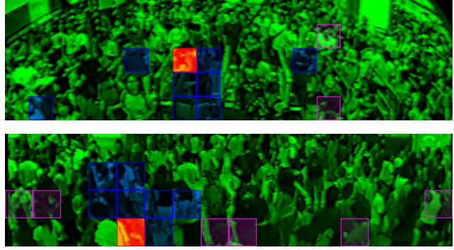
Figure 10. Pedestrians loitering or not moving in areas of high traffic are successfully detected. A few false negatives are adjacent to true positives, thus we consider them harmless in practical scenarios.
