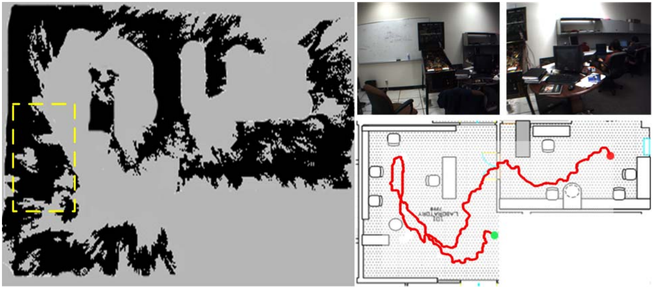
Figure 4. Indoor experiment result. The non-textured 3D map is projected onto the XY plane. Lower-right shows the floor plan of the two rooms with the camera trajectory (red) exhibiting a loop. The highlighted section on the map corresponds to the images (top-right) captured during the beginning and end of loop execution. Loop closure was detected with a probability of 0.9984.
