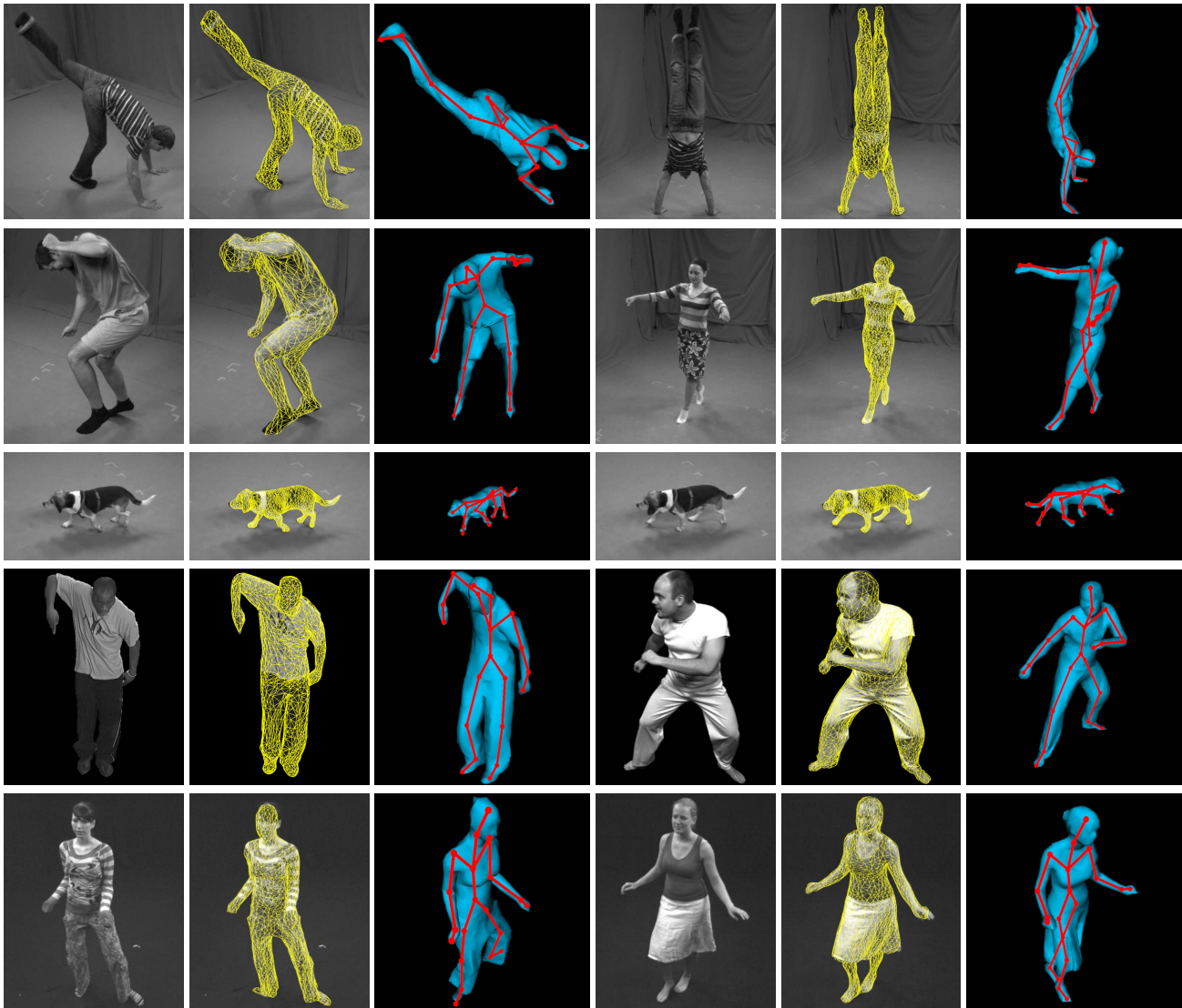
Figure 6. Input image, adapted mesh overlay, and 3D model with estimated skeleton from a different viewpoint respectively.
