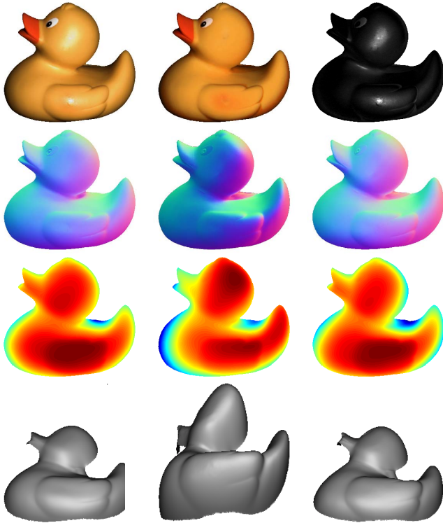
Figure 4. Resolving the GBR from a single image. Top : One input image and its diffuse and specular components. Second row : recovered normal fields, linearly-coded in RGB. Third row : depth maps from integrated normal fields. Fourth row : Reconstructed surfaces. Columns from left to right correspond to: “ground truth” obtained using calibrated sources; uncalibrated reconstruction up to a GBR; and our auto-calibrated result.
