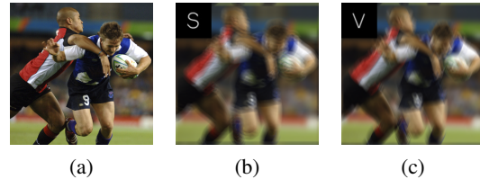
Figure 4. (a) The original clear image. (b) One blurred image. (c) Another blurred image. The corresponding blur kernels are shown on the top left of the images respectively.
