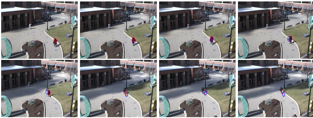
Figure 1. Tracking example on OTCBVS OSU 1b color image sequence. From left to right and top to down, the frame numbers are 1,19,32,39,121,171,184,194 respectively. Results of region covariance and SOG are marked by blue and red ellipses respectively.
