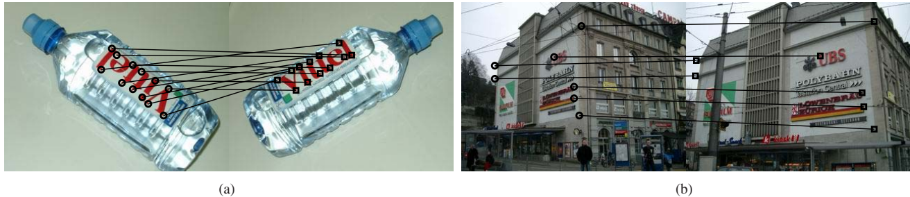
Figure 3. Examples of 2D matching for a image pair with large degree of rotation in (a), and for a stereo pair with wide baseline in (b).
