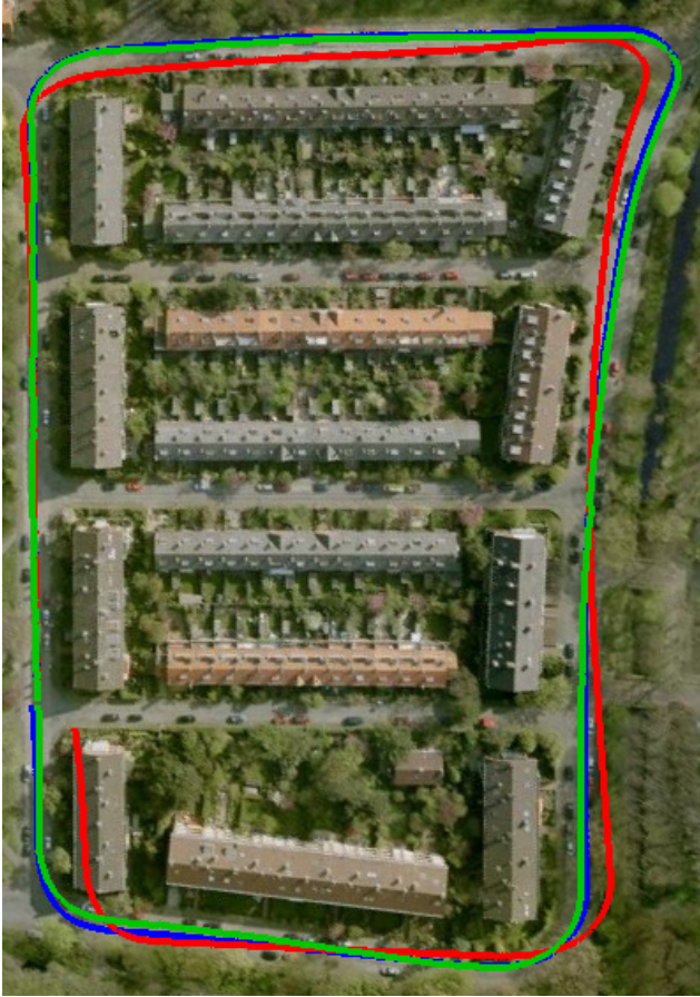
Figure 6. Calibration data-set, of approximately 800 m, used to obtain the appropriate bias gains. DGPS based groundtruth (green), HEIV on inlier landmarks (red) and HEIV using the manually tuned bias reduction technique (blue).
