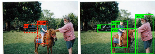
Figure 1. On the challenging PASCAL VOC dataset, even the best local-window detectors [7] often have problems with false positives, poor localization, and missed detections (left). In this paper, we enhance these detectors using contextual information (right). Only detections above 0.5 precision are shown. (Red Dotted: Detector, Green Solid: Detector+Context)
