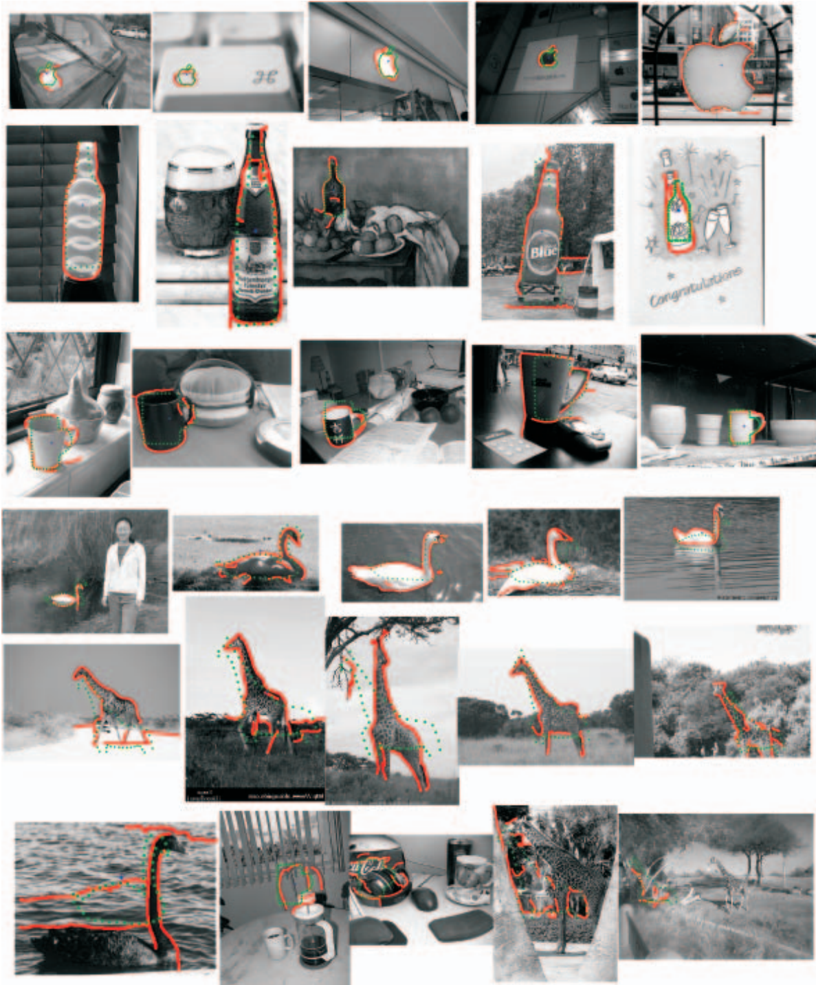
Figure 8. Selected results on ETHZ dataset [9]. The points (in green) denote the contour template, and the segments (in red) are the final obtained edges. The last row are selected worst results.
