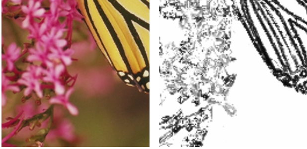
(a) A region of “Monarch,” down-sampled 2x and reconstructed. (b) The inferred PSF standard deviation \mathbf{S}^\sigma . Darker is narrower.
