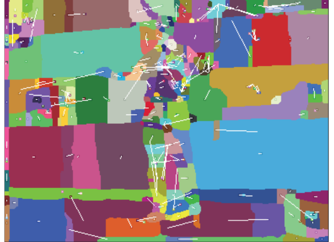
Figure 3. Displacement vectors of the matched regions drawn at their centroids. Many matches are good, but there are also outliers from regions that are not descriptive enough or their counterpart in the other image is missing.
