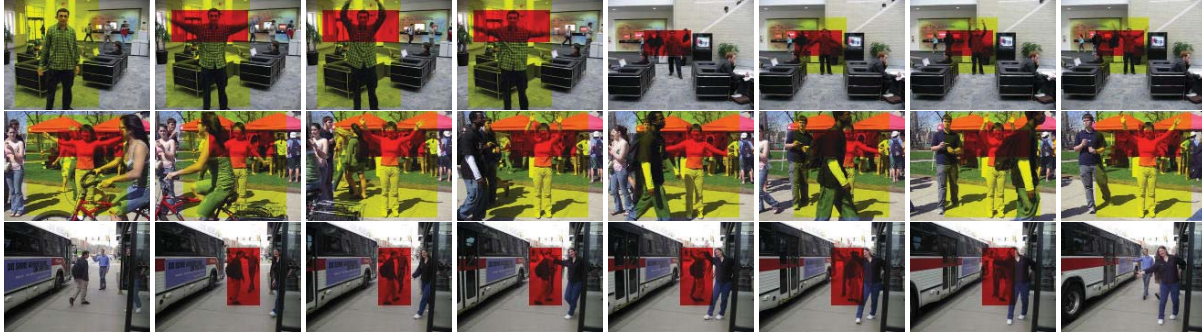
Figure 5. Detection results of two-hand waving. The yellow bounding box is the ground truth label of the whole human body action and the red bounding box is our detection of two-hand waving. The 1 st row: detection under multiple spatial scales; the 2 nd row: detection with partial occlusions; the 3 rd row: a false detection caused by two individual hand-wavings from two different persons. More results can be seen in the supplementary materials.
