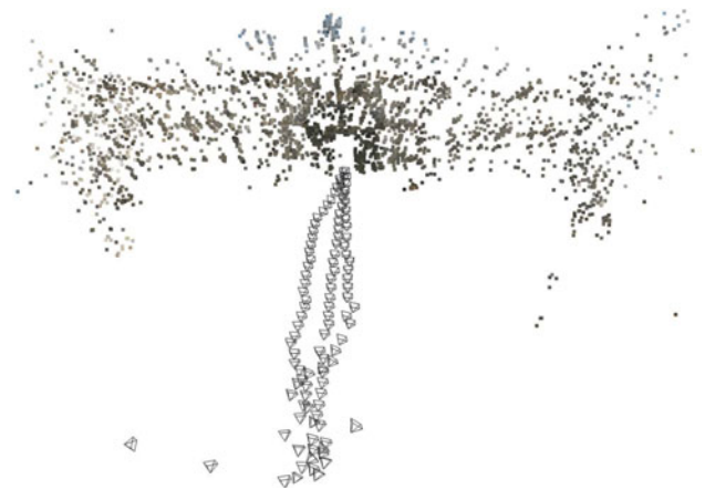
Figure 9. Partial reconstruction #471 of data set CASTLE. Entrance to the Prague Castle was reconstructed from 60 cameras, another 49 cameras were connected during gluing.
