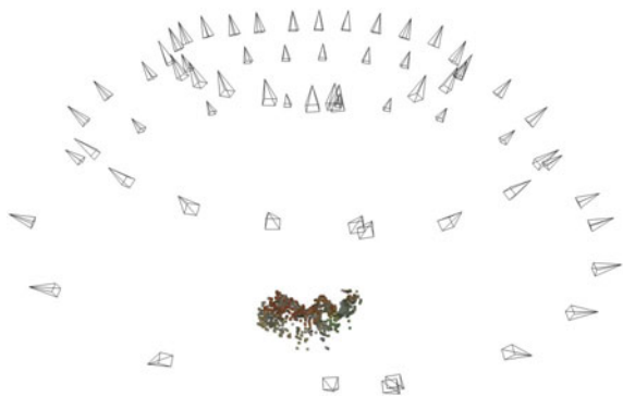
Figure 3. Complete reconstruction of data set DALIB. Partial reconstruction containing all 39 cameras from selected atomic 3D models was extended with 25 missing cameras during gluing.
