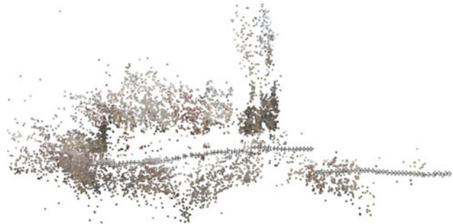
Figure 8. Partial reconstruction #407 of data set CASTLE. Part of the Old Town Square with the clock tower was reconstructed from 69 cameras, another 39 cameras were connected during gluing.
