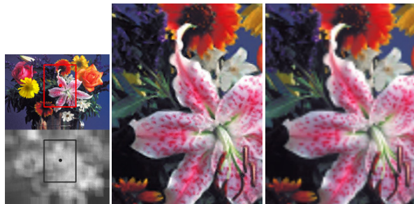
src region: 76 \times 102 pixels, dest region: 240 \times 320 pixels, scale: \times 3.15 Figure 7. Illustration of Content-Based Automatic Zooming (left: the original image and the local complexity map; middle: our results; right: BiCubic interpolation)
