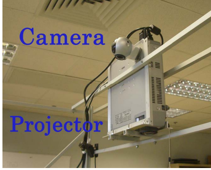
Figure 5: A projector and a webcam are fixed together to form a projector-camera pair.
