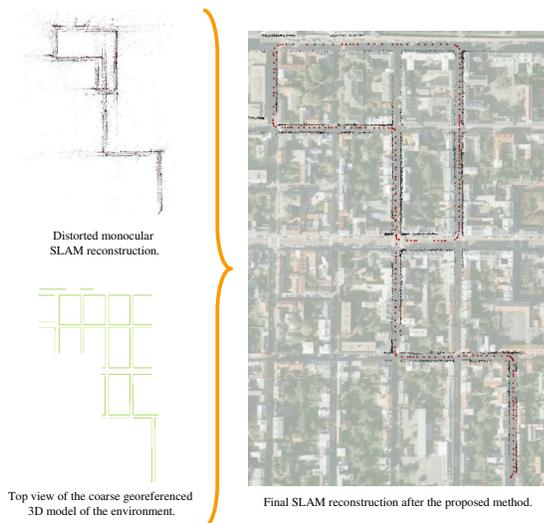
Figure 1. **Summary of the proposed method.** We proposed to correct an original distorted SLAM reconstruction thanks to a coarse 3D model of the environment. The result is superimposed on a satellite image.
