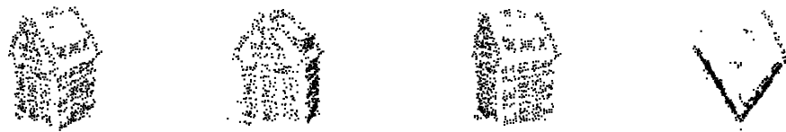
Figure 7. Reconstructed shape corresponding to the 182 image sequence shown in Fig. 5(a). The sequence consists of 816 trajectories and the missing data amounts to approximately 55%. As can be seen, the shape looks satisfactory. Due to the use of the affine camera model some angles are distorted which is shown in the fourth image (top-view).
