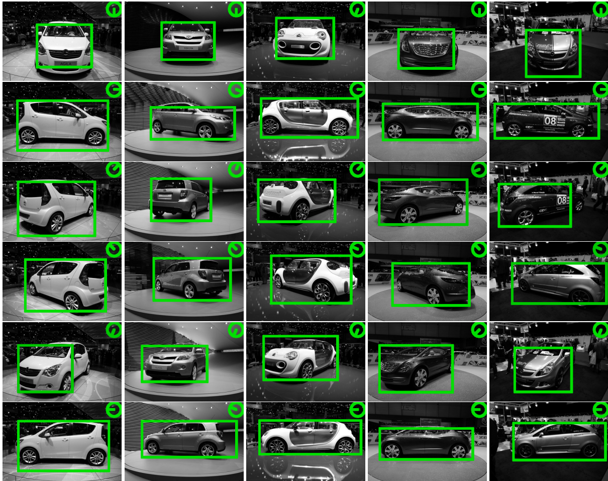
Figure 1. Sample detections from the test set. The green rectangle depicts the recovered bounding box and the estimated viewpoint is indicated inside the green circle at the top-right corner. A front facing car is indicated by a downward pointing line. Despite the challenging lightning conditions and changing backgrounds our approach can correctly localize cars and estimate their pose.
