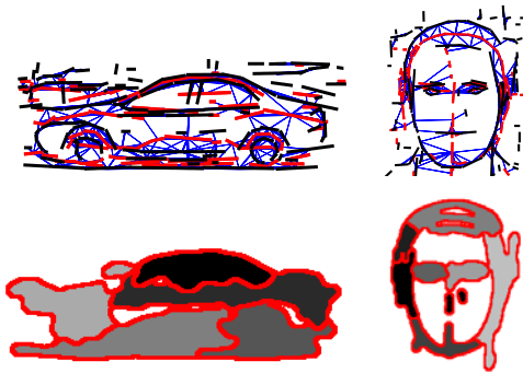
Figure 6: Top Row: Adjacency graphs among edge (black) and ridge (red) lines for cars and faces. The arcs of the graph are shown in blue and their width indicates the affinity between the lines. Bottom Row: Object parts found using spectral clustering of the adjacency graphs. (Gray-level encodes part label)
