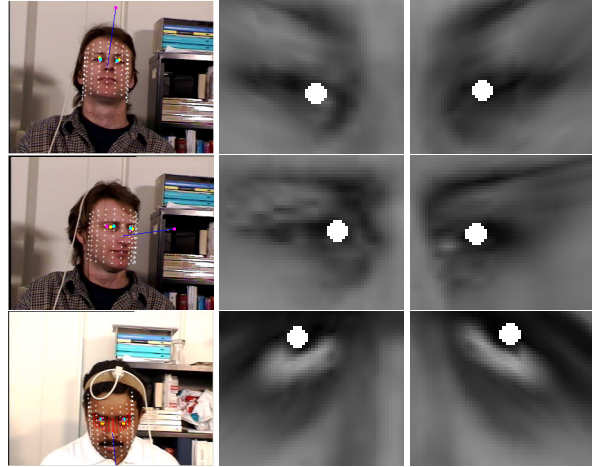
Figure 2. An example of extreme head poses and the respective pose-normalized eye locations. The results of the eye locator in the pose normalized eye region is represented by a white dot.
