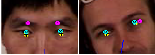
Figure 3. A mistake of the standard eye locator (.), corrected by the pose cues (x) according to the reference points (+)
