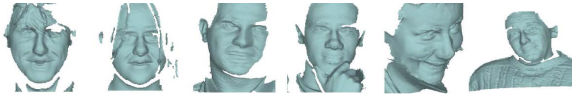
Figure 3. Sample faces with data defects from GavabDB. From left to right: 1) - 2) occlusion by hair; 3) occlusion by head rotation; 4) occlusion by hand; 5) impulse noise around the chin caused by scanning artifacts due to shading; 6) under-sampled facial area.
