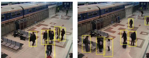
Figure 10. Illustrative detection results of the grid-based person detector for the PETS 2006 Sequence .
