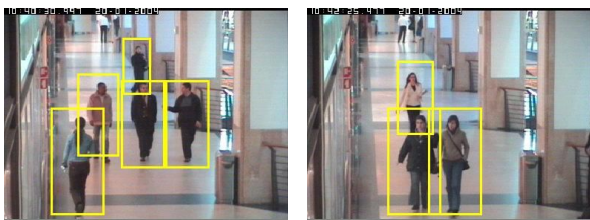
Figure 8. Illustrative detection results of the grid-based person detector for the Caviar Sequence .
