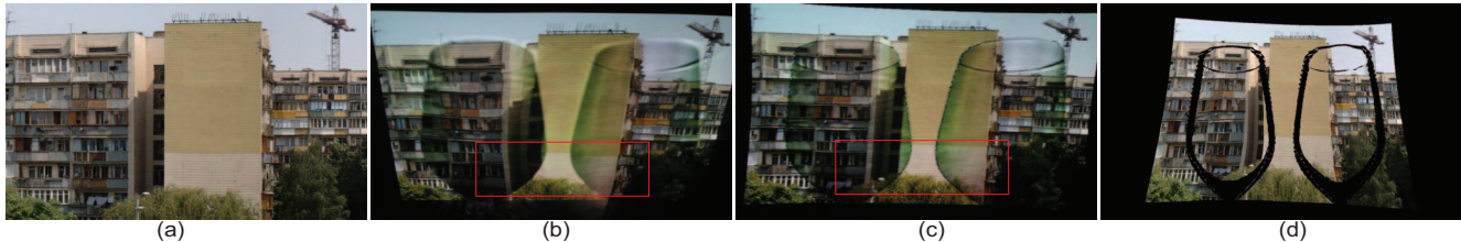
Figure 9. Close-up Views of the Wine-glasses Projector Results. (a) is the desired projection result. (b) and (c) show the projection results before and after distortion correction. (d) shows the actual projected image.
