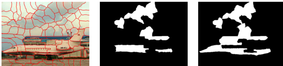
Figure 14. Image/CRF/CRF+conn. Failure case: the CRF segmentation is bad (middle) connectedness does not help (right).
