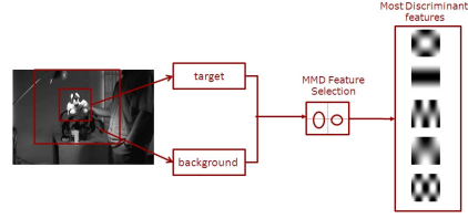
Figure 1. MMD feature selection for target/background discrimination. Feature responses are computed at the target location, from the center (target) and surround (background) windows. Features are ordered by their MD, and the most discriminant are selected.
