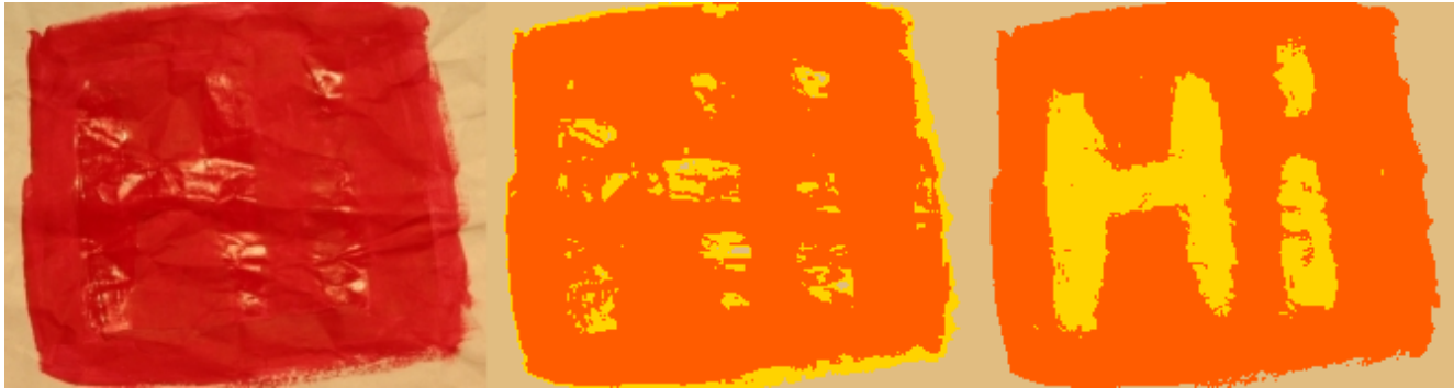
Figure 1: Capturing a BRDF slice and applying a reflectance model improves material classification. Sample captured image, 1 of 64 (left), Classification based on single image (middle), Classification based on Hemispherical Harmonic coefficients (right)
