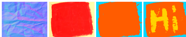
Figure 10: Per-pixel normals (left) and albedo (center-left) computed with photometric stereo. Classification results using only this data (center-right). The desired classification achieved using reflectance information (right).
