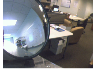
(a) Typical "ad-hoc catadioptric" frame
