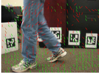
(a) Typical frame ( 640 \times 480 ) showing outlying sparse flow vectors (in red) found by our method.
