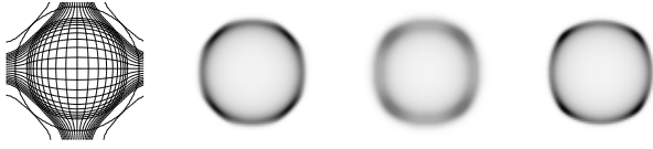
Figure 5. Determinant of Jacobian of \Phi . Left to right: Warped grid, \Phi , |D\Phi| map, |D\Phi| 1st-order, and |D\Phi| WENO5. WENO5 produces a faithful result by solving a scalar conservation law. The 1st-order approach matches qualitatively, but introduces blurring.
