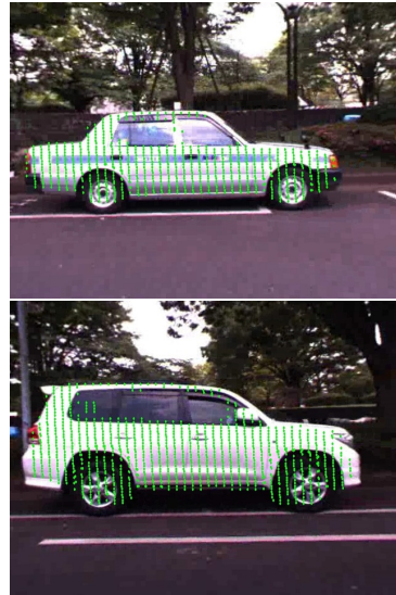
Figure 8. Some examples of laser-scanned lines projected onto the corresponding images. Scanned points are marked in green
