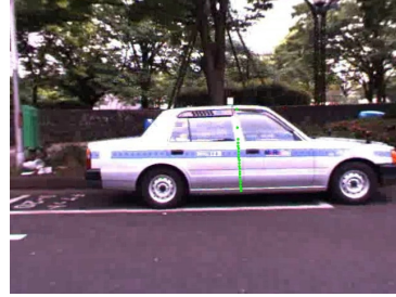
Figure 7. The points in one laser-scanned line are projected onto the corresponding image. Laser points are marked in green.
