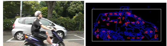
Figure 15. A successful classification of a partially occluded vehicle
