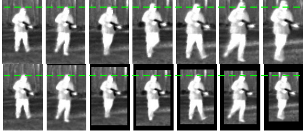
Figure 5. Example of appearance matching for a difficult sequence from the Terravic Motion IR Database[14]. Every 10^{th} frame from the original sequence (top row) and the corresponding frames registered to the first frame (bottom row). The green line shows how well the scales of all the frames match the first frame after registration. Note how the registration can robustly handle scale change, motion in the legs and even a slight rotation of the person’s head.
