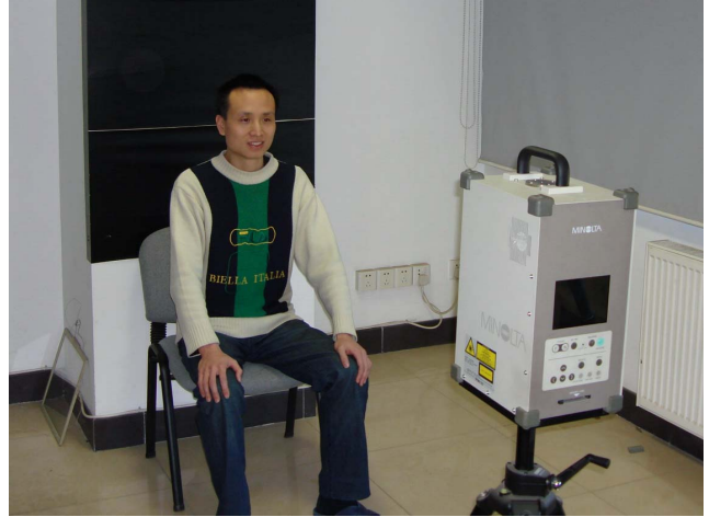
Figure 3. 3D face capture device and environment. Subjects are seated in front of black background and scanned by Minolta vivid 910 laser scanner.
