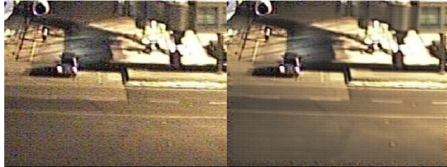
Figure 8. A noisy webcam image, and a version with noise reduced using non-local (temporal) averaging.
