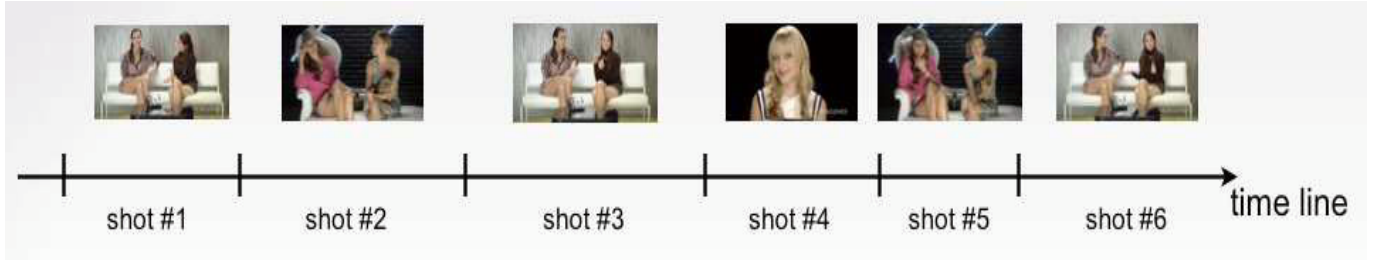
Figure 2. Example of shot clustering within a video. A video is composed of consecutive shots. A representative frame for each shot is shown above the timeline. Notice that shots 1,3,6 are all similar and shots 2,5 are similar as well. Our shot grouping algorithm, as described in Section 2.4 should group together these shots.
